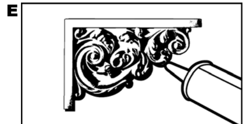
Apply paintable caulk around edges
